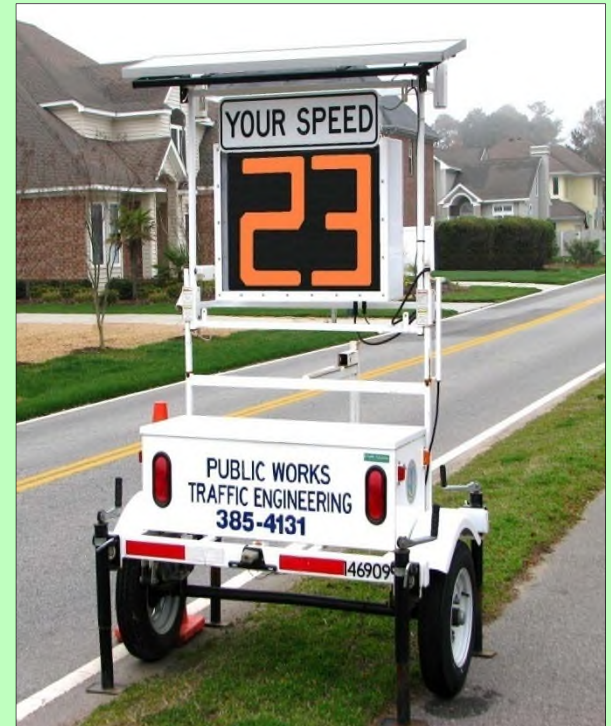
Speed Trailer used in Traffic Calming Program
