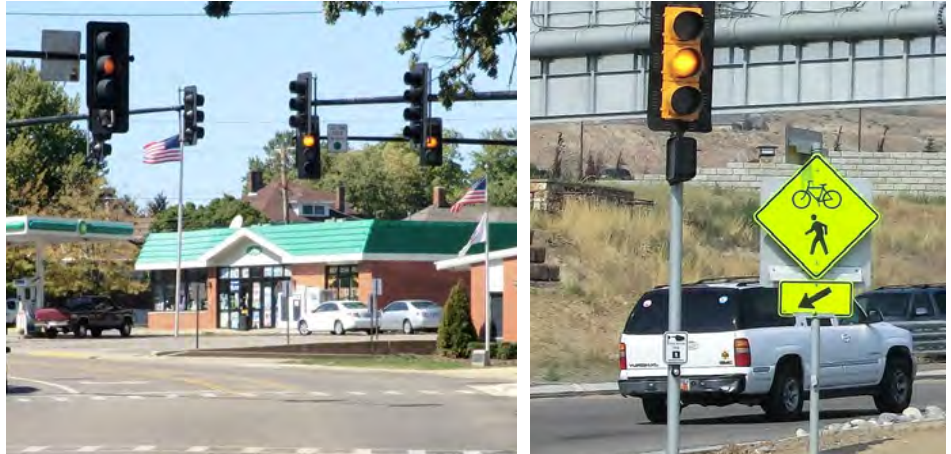
Properly-timed yellow change intervals can reduce red-light running and improve overall intersection safety.
