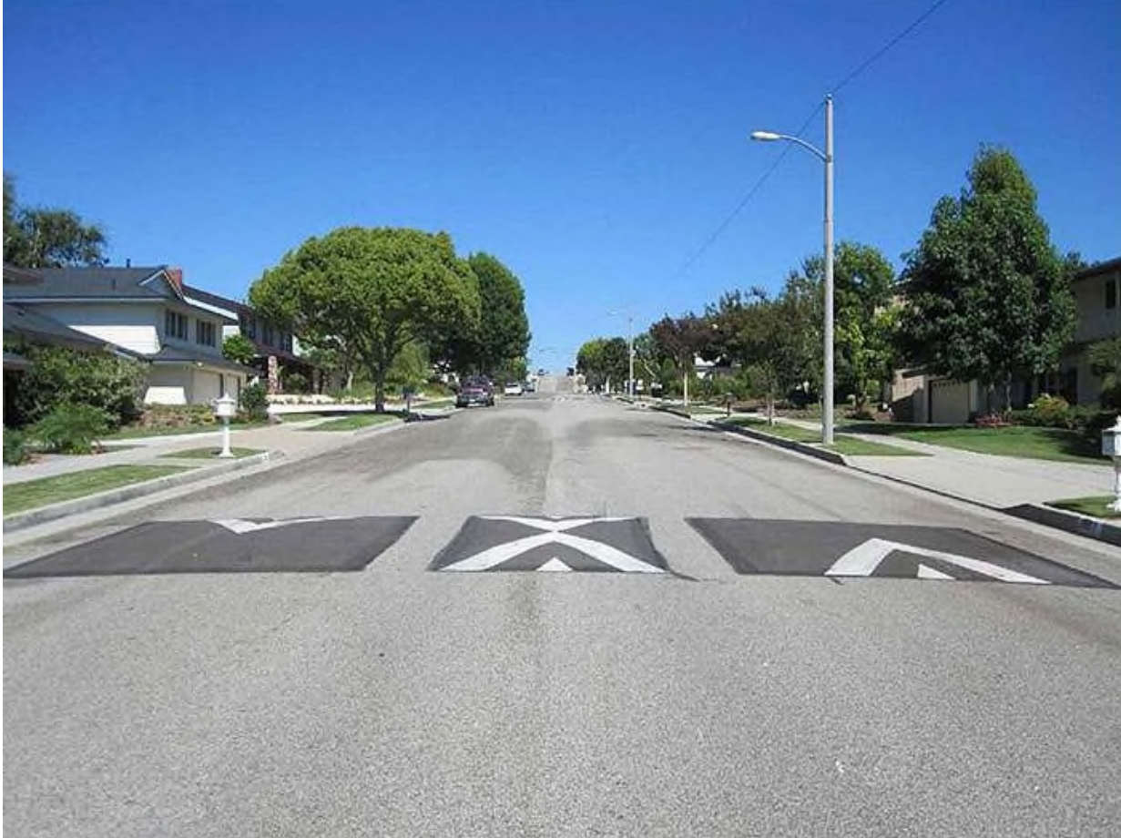
Figure 3.2. Vertical Deflection Measure – Speed Cushion (Source: FHWA Module 1-Jeff Gulden)
